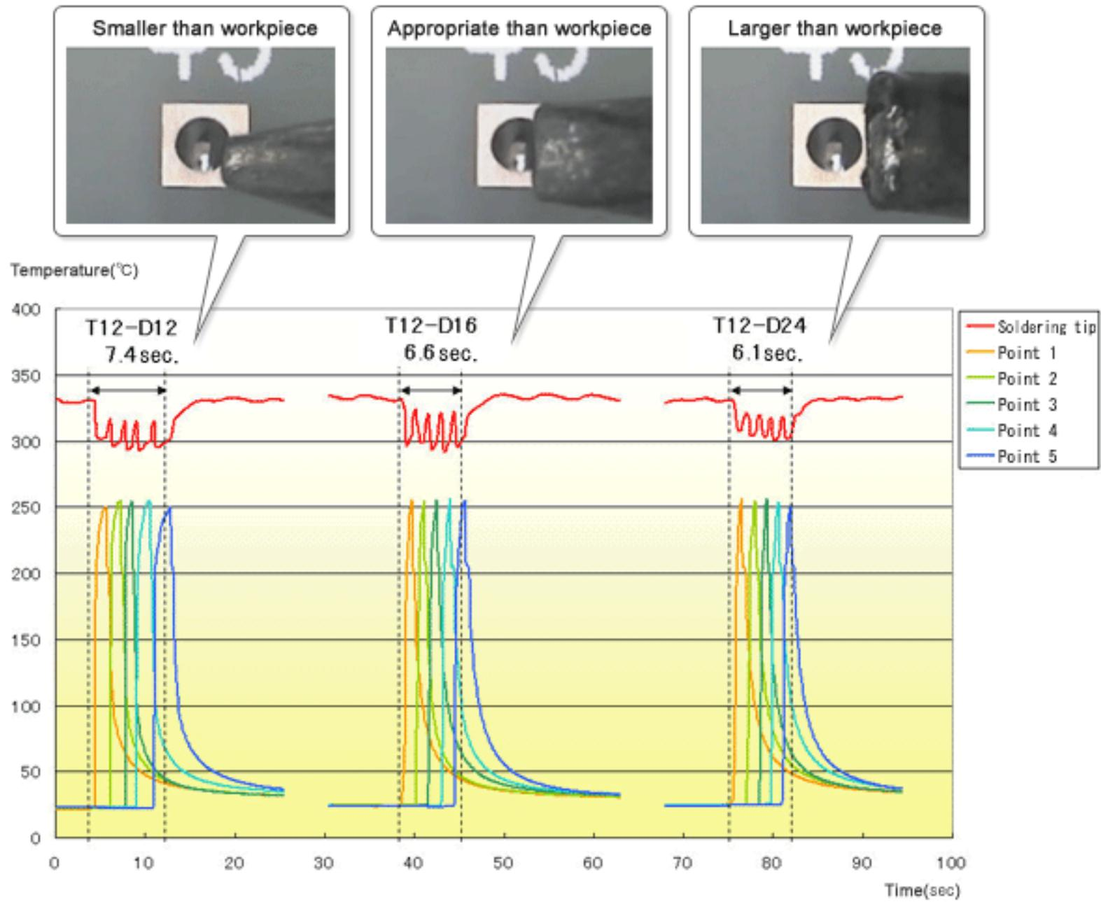
Figure 1. Select a tip with the appropriate size for the work piece
