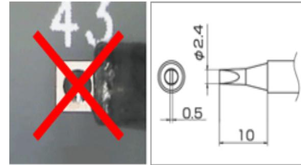
Do not use a tip larger than the workpiece.
