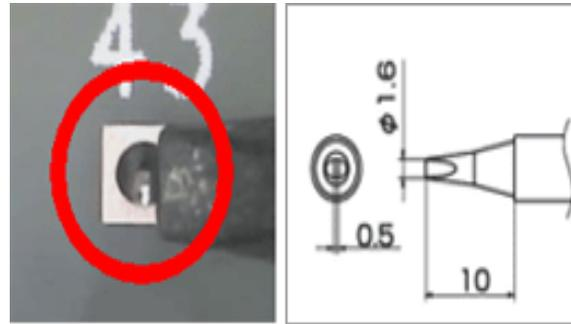
A tip with the appropriate size for the workpiece can transfer heat to the workpiece efficiently
