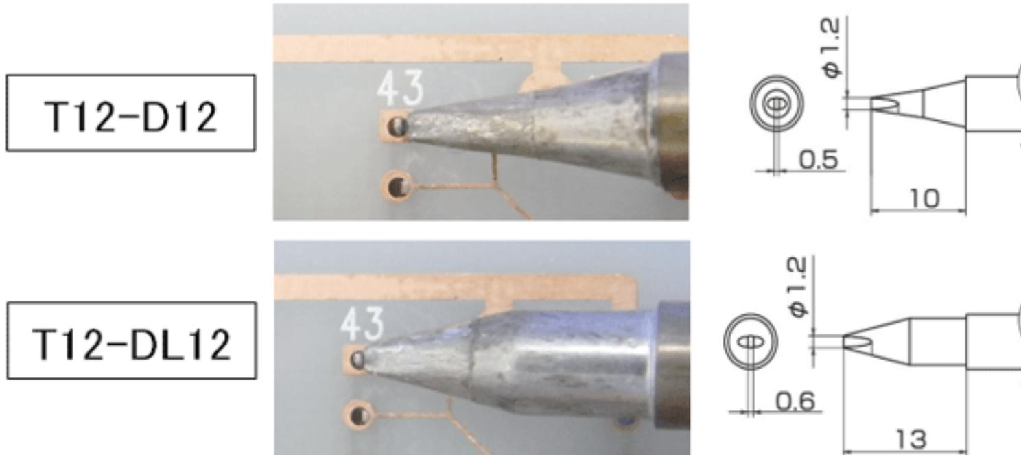
\* Although the tip size is the same for both, the heat storage capacity is different
