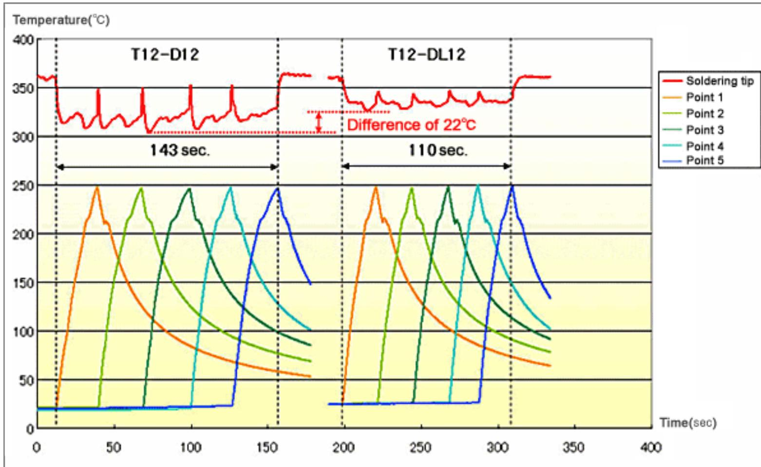
Figure 2. Select a tip with as high a heat storage capacity as possible
