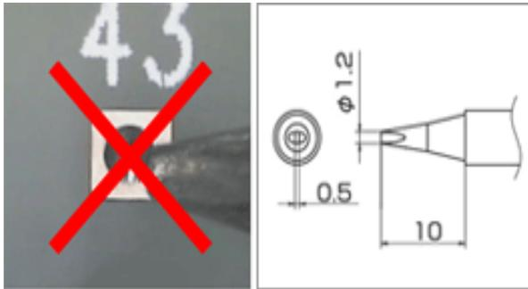
A tip smaller than the workpiece cannot transfer sufficient heat to the workpiece
